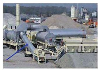
FIGURE 5: EXEMPLE DE CONVOYEUR A BANDE POUR L'ALIMENTATION DU TAMBOUR (ERMONT ©).
