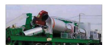
FIGURE 6: EXEMPLE DE TAMBOUR-SECHEUR-MALAXEUR (ERMONT©).
